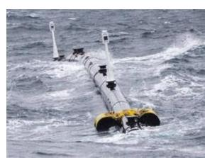
A two-week test of the collection system's durability and hydrodynamics showed it withstanding the forces of the Pacific Ocean, including 5-meter (16.4 feet) wave.
