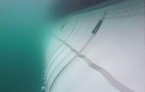
This woven polyster screen is an important component of The Ocean Cleanup system. Attached to the buoyant "floater" of polyethylene pipe, the drag on the tapered screen forms a U-shape retention area that captures plastic floating at or near the surface.
